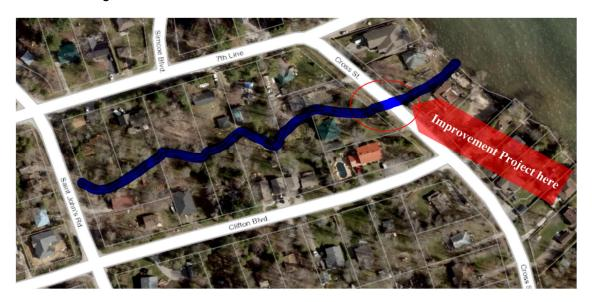
Throughout the design phase, it has been determined that the issues relating to flooding, direction of water and property access would only be slightly improved by moving forward with the preferred alternative of replacing the culvert structure which is in good condition.
