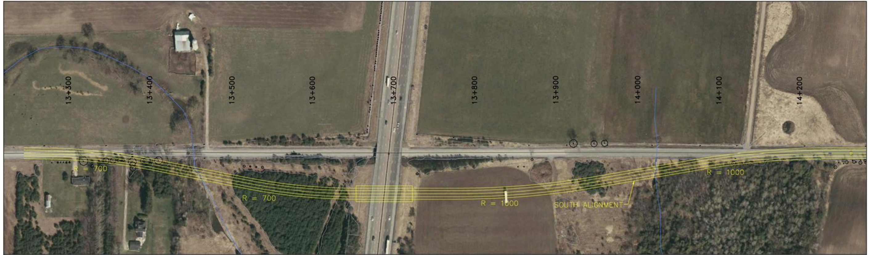
Figure 5.4: Horizontal Alignment Alternative C (not carried forward)
