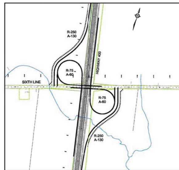
ALTERNATIVE 3 PARCLO A2 180m DIRECT TAPER ON SIXTH LINE (100 km/h DESIGN SPEED)
