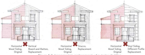
Figure 5-3: Inappropriate replacements of exterior cladding
