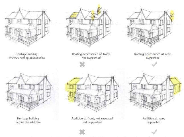
Figure 5-6: Additions, Dormers, and Roof Accessories, Examples not Supported
