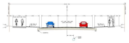
Reconstruct this segment to a 3 lane urban cross-section providing:
