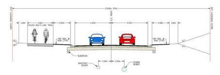
Reconstruct this segment to a 2 lane urban cross-section providing:
