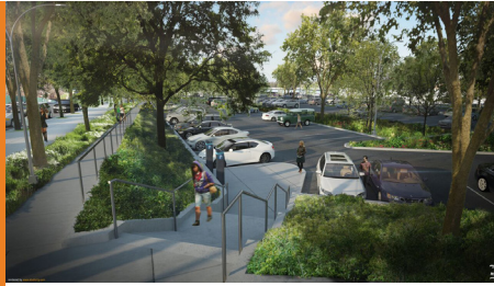
Figure 1-51 Green retrofit parking lots are an opportunity to update space and lane widths with narrower modern standards, integrate safe passage for pedestrians, and incorporate LID.
